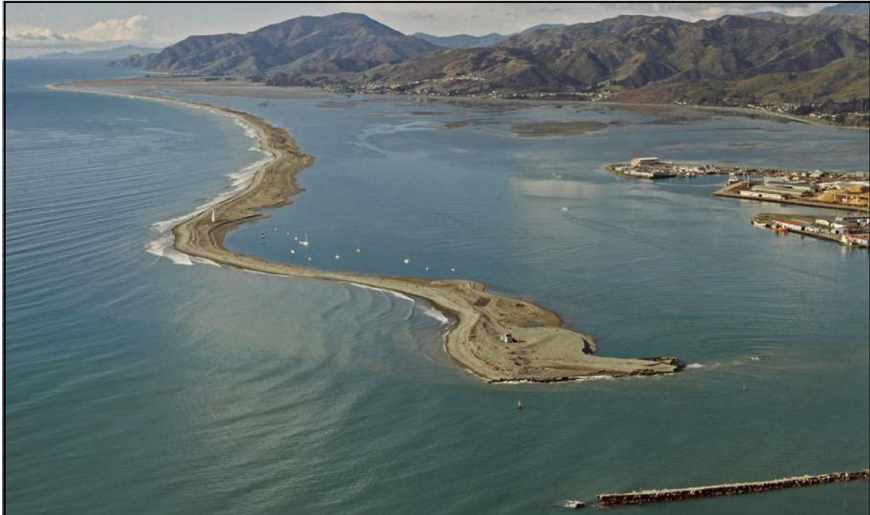
Fig. 22.8. 11-km-long Nelson Boulder Bank was mostly formed by southwest longshore transport of gravel from its source around Mackay Bluff when sea level was near its present height in the last 7000 yrs. Photographer Lloyd Homer, GNS Science.
