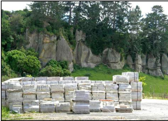
Fig. 7.3. Bluffs of welded ignimbrite at Hinuera are sawn into blocks for use as a building stone. Photographer Adrian Pittari.
