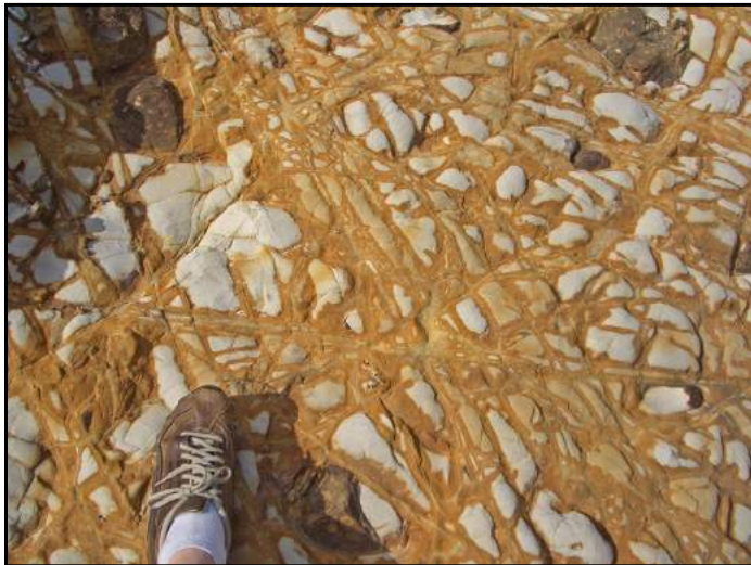
Fig. 6.4. This weathered greywacke rock on Rotoroa Island, Hauraki Gulf, is cut by numerous near-vertical joints (cracks). Chemical weathering has produced the orange iron-oxide bands along each joint. Photographer Bruce Hayward.
