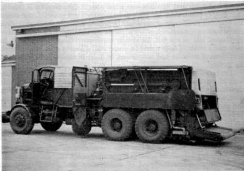
Fig 6. High speed road surfacing unit
