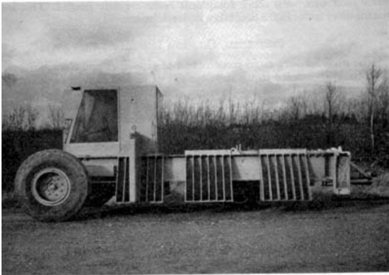
Fig 7. Airfield pavement test trolley
