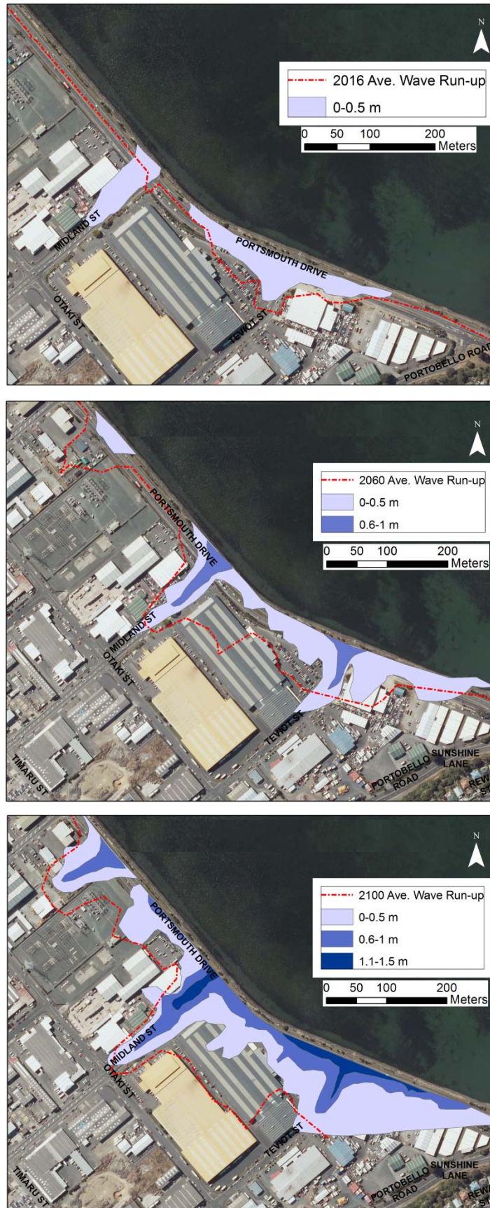
Figure 44. Likely extent and depth of inundation (shaded areas) and maximum extent of wave run-up (red-line) from Otago Harbour during a 1:20-year storm surge event at MHWS. Current sea level (top), 0.3 m mean sea level rise (middle), and 0.5 m rise (lower). Ave = average.
